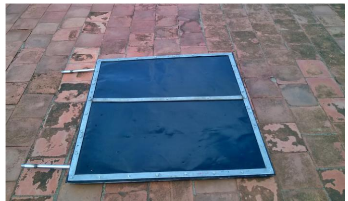
(c) Inner tray with black paint coated copper cover
